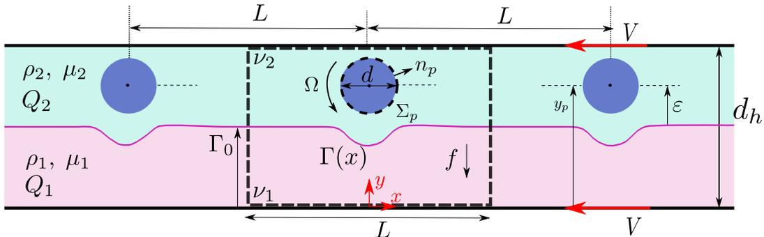
FIG. 1. Schematics of the flow configuration, including the geometrical and fluid-dynamical relevant parameters.
